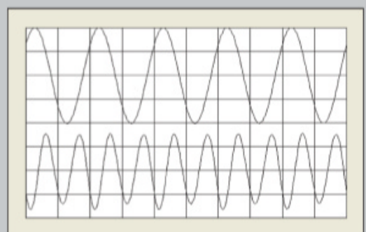
Fig.13 Cary CAD-805RS, 845 tube, 0dB feedback, 4 ohm tap, 1kHz waveform at 1W into 8 ohms, 0.284% THD+N (top); distortion and noise waveform with fundamental notched out (bottom not to scale).
