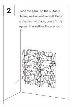
To ensure that you maximise the strength of the glue, don't make any adjustments to the panel after bonding
