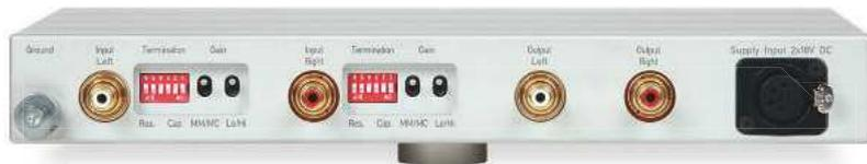
**ABOVE:** Input/outputs are via WBT Nextgen RCAs, loading via DIP switches and MM/MC gain via toggles
