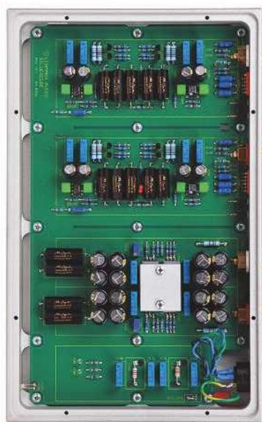
**ABOVE:** Mundorf tin foil and mica caps feature in the dual-mono eq and input amps, the latter using mic-grade op-amps
