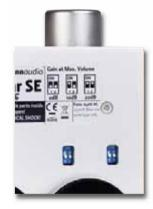
Via the dip switches the gain factor can be raised by up to 20 dB, e.g. for magnetostats
